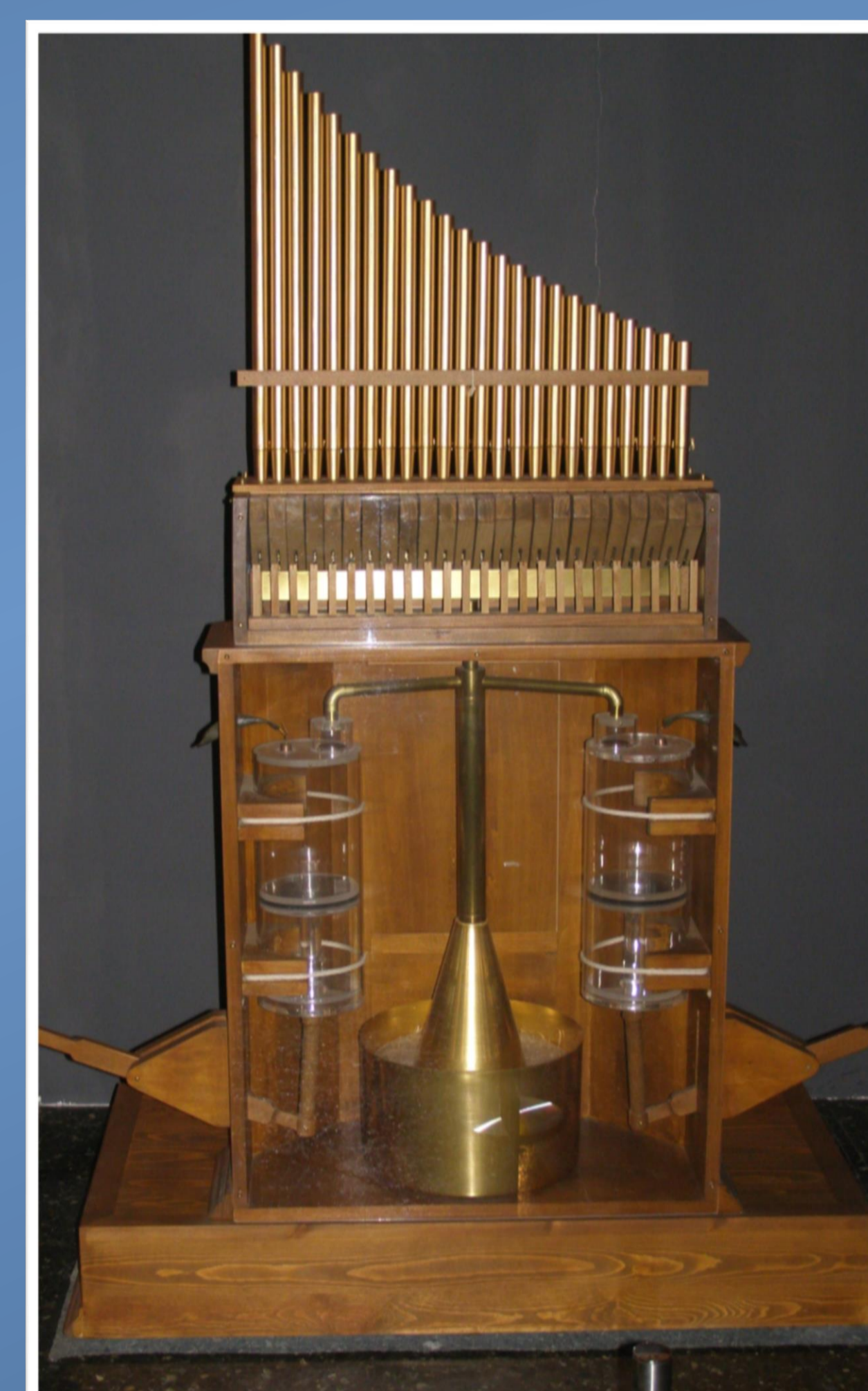
2. Reconstruction of hydraulis in the the Traveling Exhibition of Kotsanas Museum of Ancient Greek Technology
