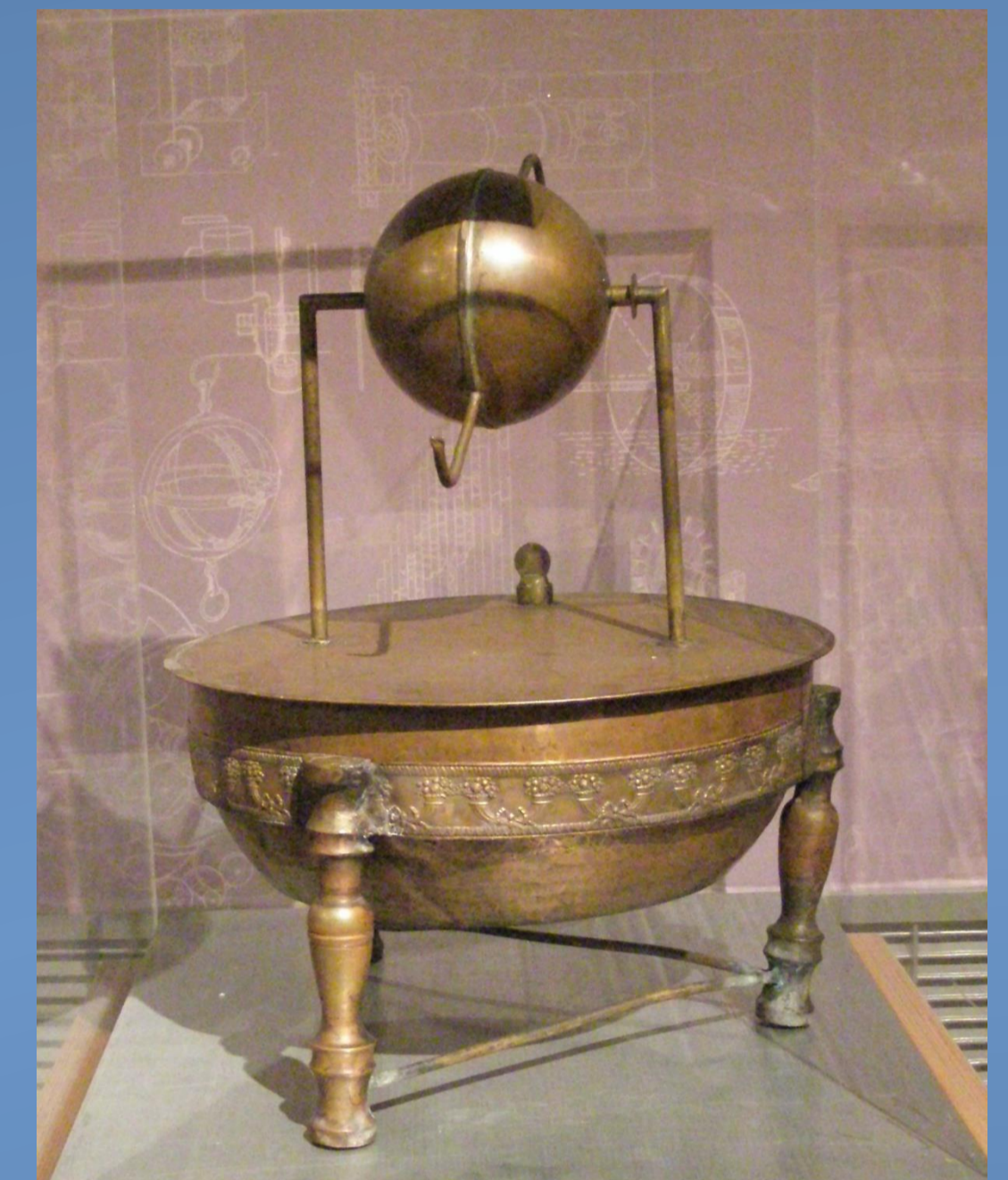
7. Heron's aeolipile was a more archaic version of a steam working machine.
