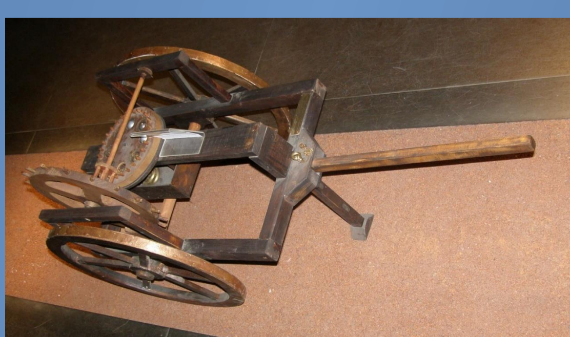
3. The odometer : Heron describes how the wheels on chariots could be used as a car odometer
