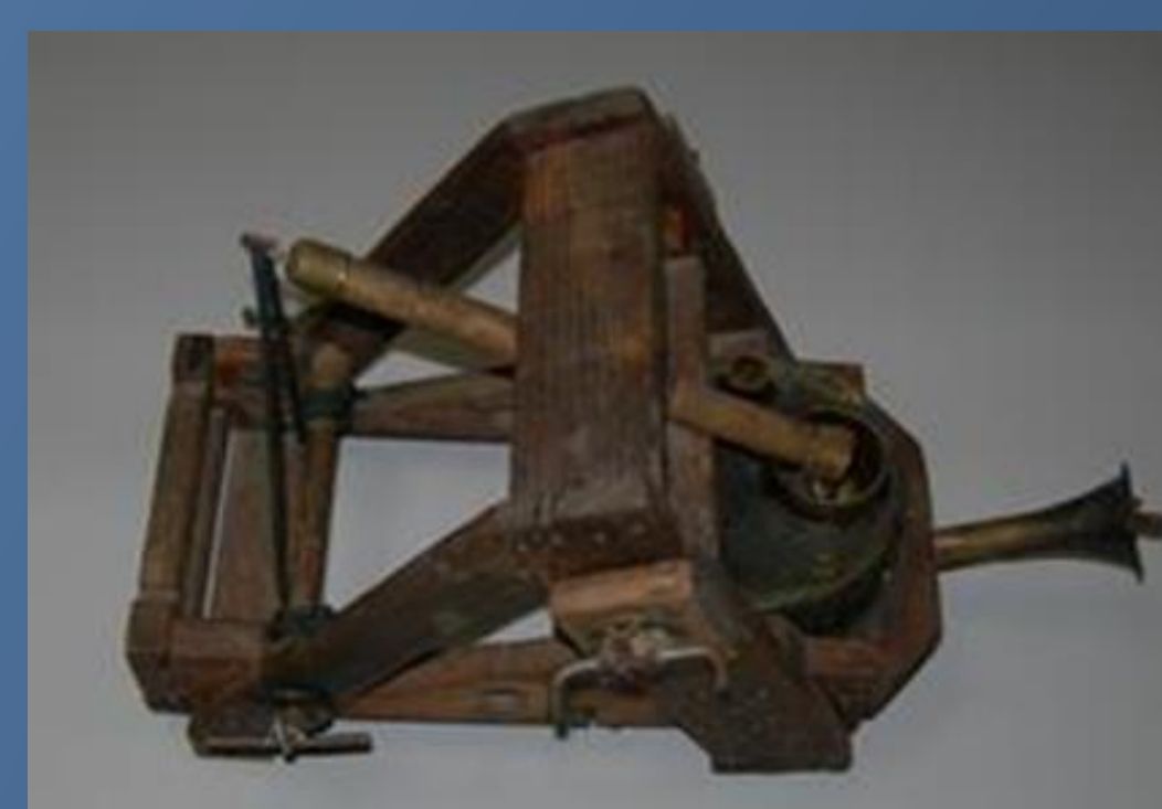
6. Strepton was a union of a catapult (as a source of power) and a force pump, an invention of Heron. The combination of these two mechanisms had as a result the creation of a firefighter, which launched Greek fire (Egrou Pyr), something like naphtha, in a distance of about 30m.
