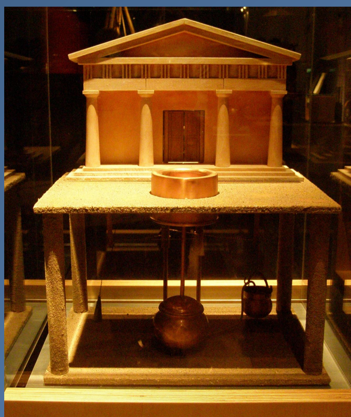
1. Heron invented the first known automatic opening and closing doors . His famous application used heat from a fire lit by the city's temple priest under the altar. After a few hours atmospheric pressure built up in a brass vessel causing it to pump water into adjacent containers. These containers acted as weights that, through a series of ropes and pulleys, would open the temple's doors.
